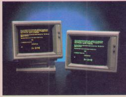
MODEL 116 12 inch High-Res Amber Monitor. Long Persistance Phosphor with non-glare screen. Fully compatible with Apple, IBM and most other personal computers. 1000 line resolution. More than 20 MHz bandwidth. 2000 character display. Optional Tilt/Swivel Base available Model 110-12 Green Phosphor available (Model 115).
